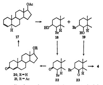
responding bromo ketones  $23^7$  (mp 152–154°;  $[\alpha]$ D – 131.4°) and 22 (mp 171–172°;  $[\alpha]$ D – 98.8°). Treatment of both bromo ketones 22 and 23 with Li<sub>2</sub>CO<sub>3</sub> afforded respective enones 21 and 4. The former enone 21 was proved to be testosterone acetate.
